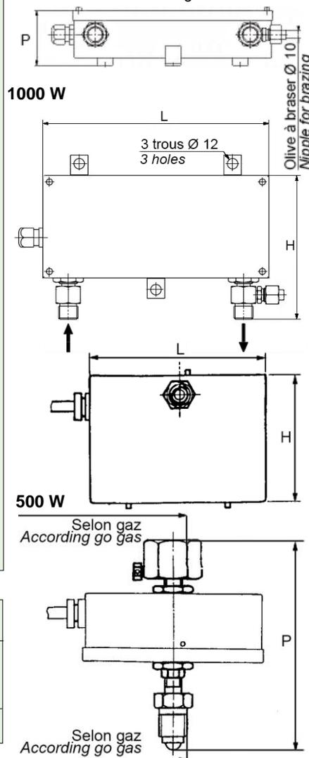
Heaters are designed for warming up high- or low-pressure medical gases (O<sub>2</sub>, mixture O<sub>2</sub>/CO<sub>2</sub> and N<sub>2</sub>O\*).
