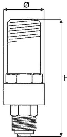
The GAUTHIER safety valves enable, by a direct mounting on a pipeline system, a pressure vessel or a hydrogen container, the evacuation of any accidental overpressure.
