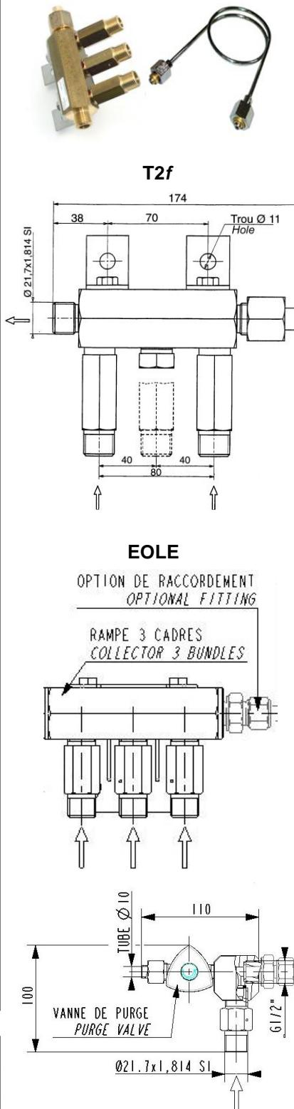
The CAHOUET HP collectors, the HP joining pipes, the HP hoses and the HP pigtails make up a complete and outstanding collector and liaison system between the cylinders or the bundles and the starting point of the gas pipeline distribution system (change-over unit, central supply panel or pressure regulator).
